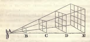
at C—they will be so much farther diffused as to occupy four such surfaces:—at treble the distance, or at D, they will be so much farther separated as to occupy nine such surfaces:—while, at quadruple the distance, or at E, they will have become so scattered as to spread themselves over sixteen such surfaces—and so on forever.
